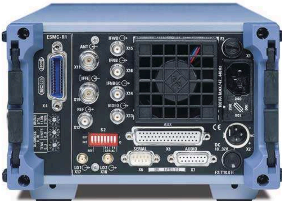
Rear of ESMC; the IEC/IEE bus can optionally be replaced by RS232 and RS422/RS485 interface
